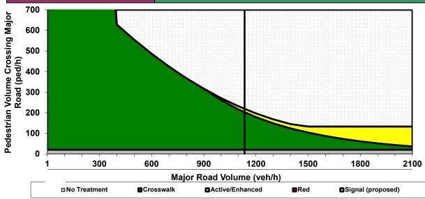
This spreadsheet combines Worksheet 1 and Worksheet 2 (Appendix A, pages 69-70) of TCRP Report 112/NCHRP Report 562 (*Improving Pedestrian Safety at Unsignalized Intersections*) into an electronic format. This spreadsheet should be used in
