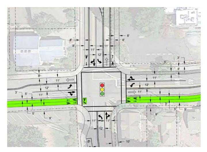
FIGURE 1.  $13^{\text{TH}}$  STREET/ MAY STREET SIGNALIZED INTERSECTION CONFIGURATION
