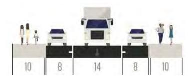
Figure 7: Revised typical street cross section for A Street (looking west).
