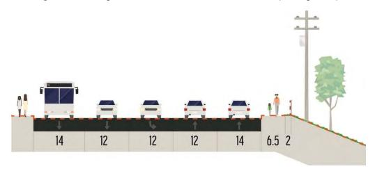
Figure 17: Existing 12<sup>th</sup> Street cross section south of Nix Dr (looking north)
