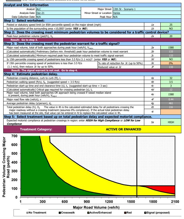
This spreadsheet combines Worksheet 1 and Worksheet 2 (Appendix A, pages 69-70) of TCRP Report 112/NCHRP Report 562 (Improving Pedestrian Safety at Unsignalized Intersections) into an electronic format. This spreadsheet should be used in
