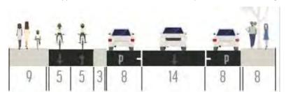
Figure 6: Revised typical street cross section for Taylor Avenue (looking east).
