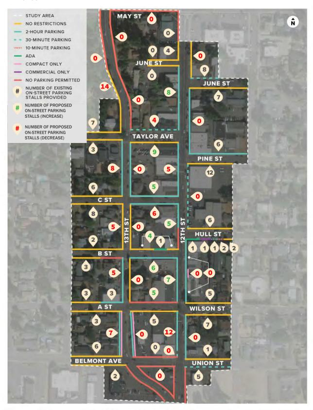
Figure 2: Planning level estimate for potential future on-street parking for recommended design (as of design studies completed March 2023)
