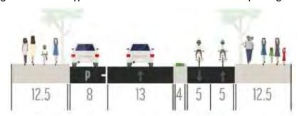
Figure 2: Revised typical street cross section for 12th Street (looking north).
