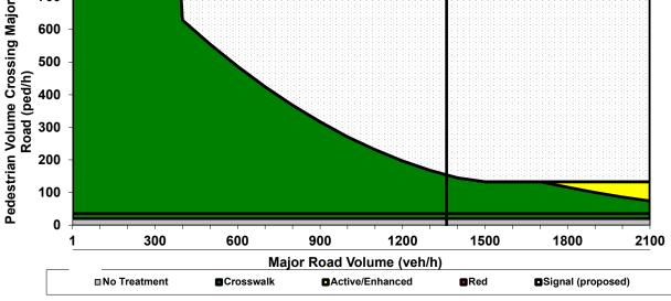
This spreadsheet combines Worksheet 1 and Worksheet 2 (Appendix A, pages 69-70) of TCRP Report 112/NCHRP Report 562 (Improving Pedestrian Safety at Unsignalized Intersections) into an electronic format. This spreadsheet should be used in
