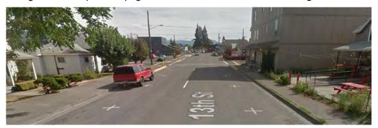
Where these existing constraints prevent the sidewalk from being widened to 10-feet (including curb) the project team recommends the city and agency explore opportunities to require building setbacks or sidewalk easements as properties redevelop so the existing five-foot sidewalk can be widened to 12-feet.
