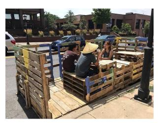
Parklets should avoid corners and are best placed at least one parking space away from the intersection corner. Where installation of a parklet is under consideration for a site near an intersection, volumes of turning traffic, sightlines, visibility, and daylighting should be taken into account.
