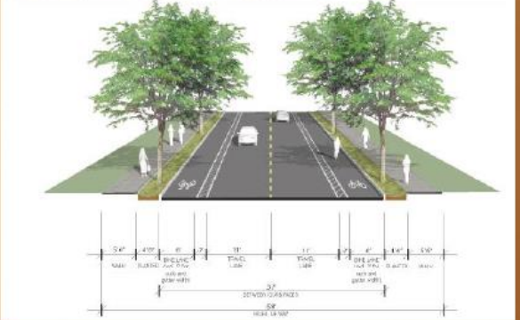
Figure 14. Minor Arterial Option Cross-Section (Without Turn Lane)
