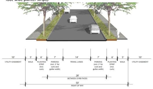
• The Commission supports incorporating traffic calming measures on 30<sup>th</sup> Street north of May Street to slow and limit cut-through traffic by the use of a narrower cross section and specific design features identified in the Concept Plan Report (see examples below). The specific methods and locations of traffic calming measures should be determined by the City Engineer as needed.
